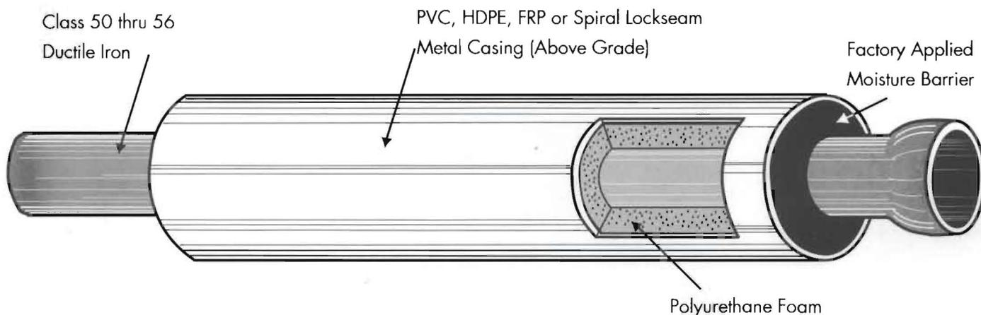
The INSUL-TEK® Ductile Iron system utilizes a tough and corrosion-resistant Ductile Iron carrier pipe conforming to ANSI/AWWA C151/A21.51. Ductile Iron Pipe offers the advantages of having the physical strengths of mild steel and the longevity of gray iron. Once insulated with our most thermally efficient polyurethane foam and protected with one of our non-corrosive protective casings, this system is an extremely tough and durable alternative to standard steel or plastic piping systems.
