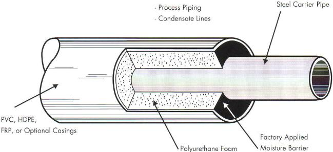
The INSUL-TEK® 250 Steel System is intended for use on systems ranging in temperature from -350° F to 250° F. It is suitable for use above and below ground. INSUL-TEK® 250 Steel utilizes the most energy efficient insulation available today, isocyanate polyurethane foam.
