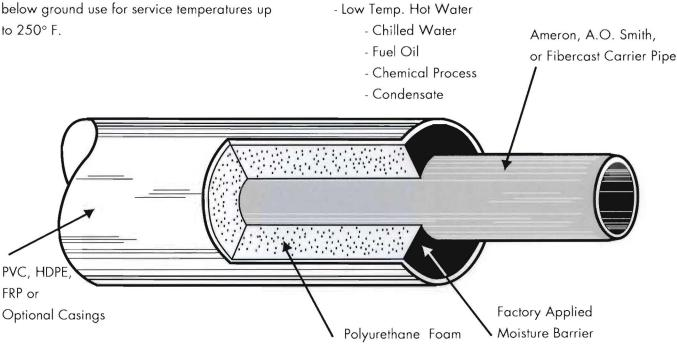
The INSUL-TEK® 250 FRP system is intended for use on systems with service temperatures up to 250° F and maximum pressures up to 150 psig. It is suitable for use above and below ground. INSUL-TEK® 250 FRP utilizes the most energy efficient insulation available today, isocyanate polyurethane foam.
