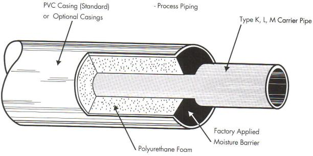
The INSUL-TEK® 250 Copper system is a totally factory fabricated, insulated and jacketed system supplied in 20' lengths. The isocyanate polyurethane foam insulation utilized in this system is the most thermally efficient type of insulation available today, making this system ideal for use on both cold and hot applications.
